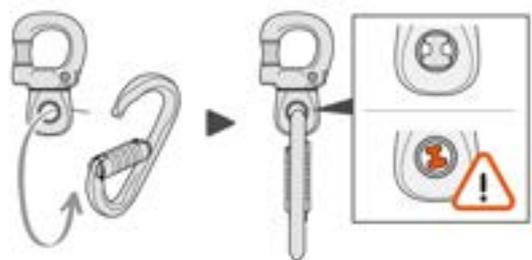
**7. Installing the swivel connector
